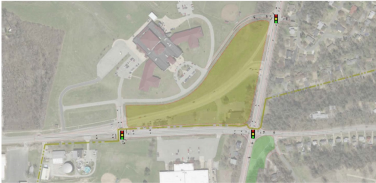
An at-grade roadway design at the intersection of St. Louis Road and Highway 157 and the relocation of a signalized intersection.
