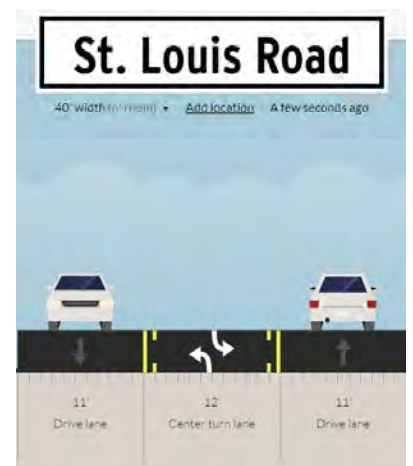
IDOT Restriping Configuration
