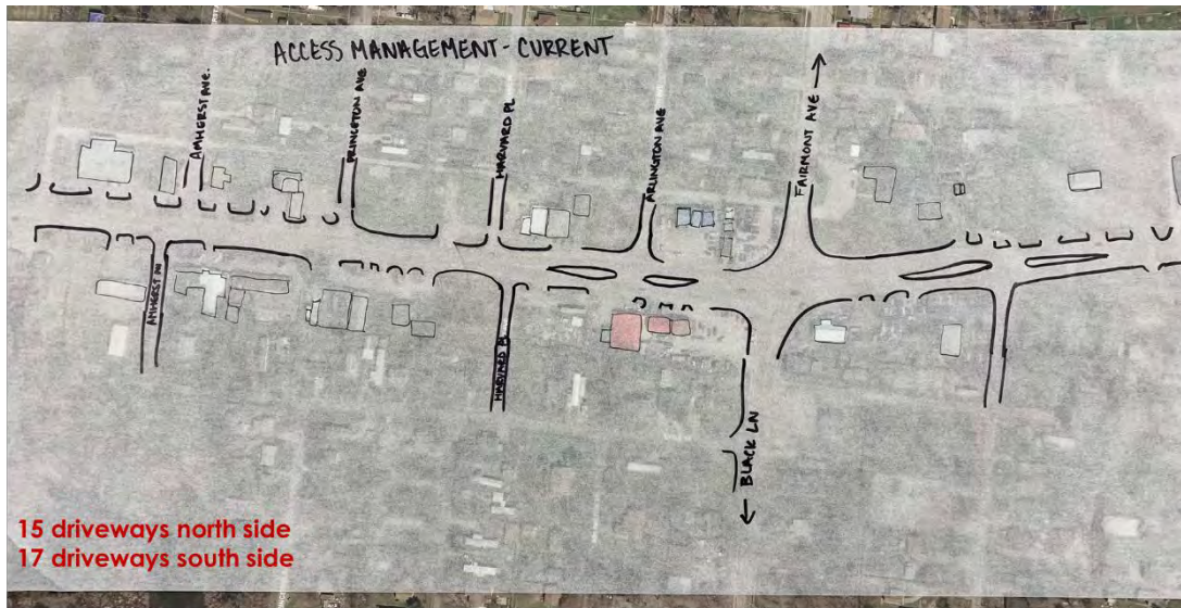
Current access management (Collinsville Road at Black Lane)
