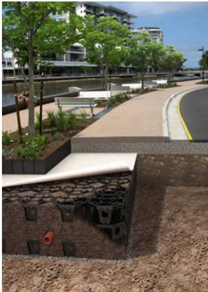
Example of a propriety structural soil system (Strata Cells). The structural cells provide support for pavement
