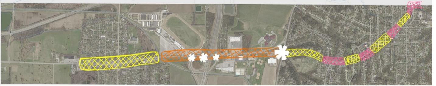
Map of proposed lighting locations. Pink: Commercial node lighting, Yellow: Residential lighting, Brown: High mast lighting, Symbols: Gateway lighting locations.
